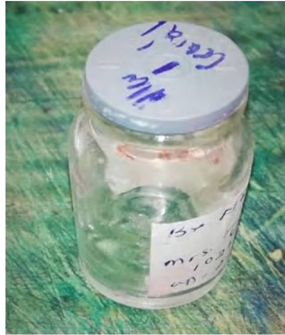
Figure 5. An unsuitable container for a small specimen with a lid that can be easily dislodged. The specimen is labelled on the lid, which should not be done.
